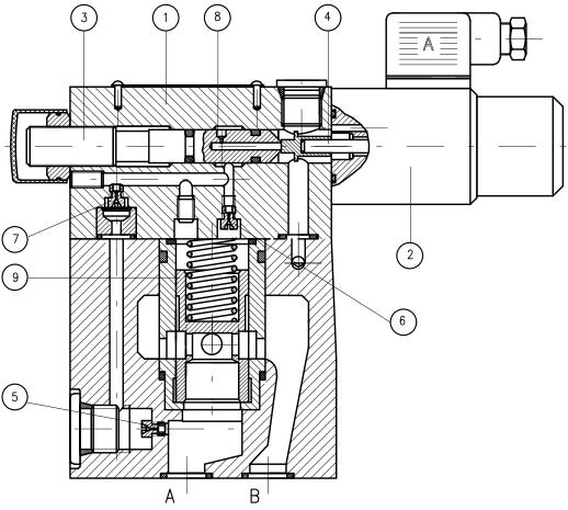
Pressure reducing valves WZRPE consist basically of the pilot unit housing 1, proportional solenoid 2, adjusting jet 3 and blind 4 connected with the proportional solenoid core. Pressure at port A acts through the system of jets 5, 6, 7, 8. On the bottom and top sides of the valve poppet 9 and blind 4 connected with the proportional solenoid core. Push force of the blind 4 to the jet 3 is
